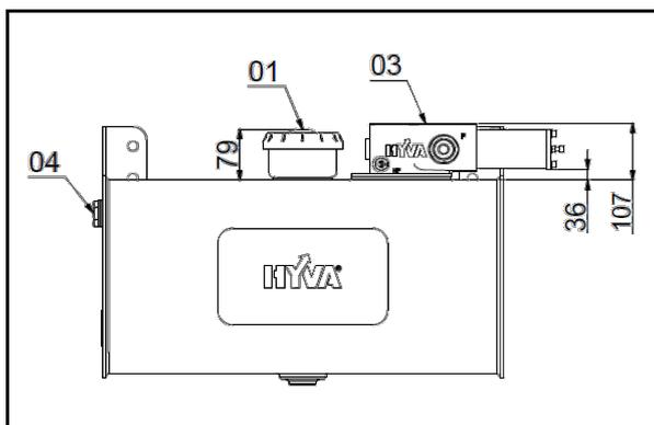
**Valve mounted on tank**
